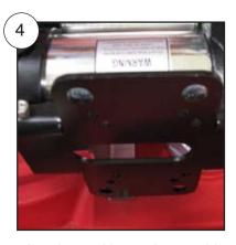
Attach metal base plate to side of pump. This will be to secure nozzle holster
