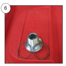
Insert Viton O rings (BS136) to grooves on both sides of coupling (400LP-C2)
