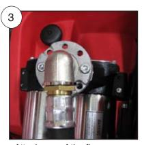
Attach one of the flanges provided to inlet of pump
